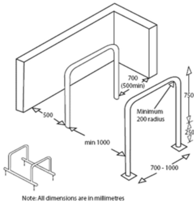
**Figure 37. Constructive dimensions of arched (n-shaped) rack, “Parking Standards”, 2005**
